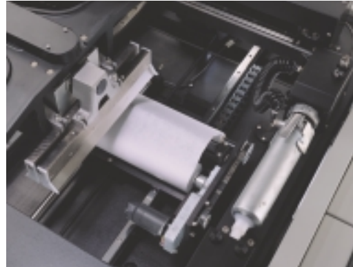
Top view featuring print head, wiper and dispenser
